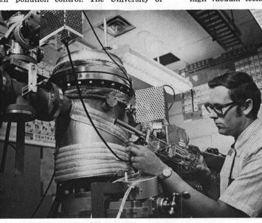
CLEAN AIR TOOLS? - Among instruments and technologies in use at Sandia that could have application in air pollution detection are the mass spectrometer (left) and the atomic absorption spectrometer. At Left, Dick Meyer (5224) prepares to install an electron multiplier detector in the mass spectrometer. Similar but smaller instruments
